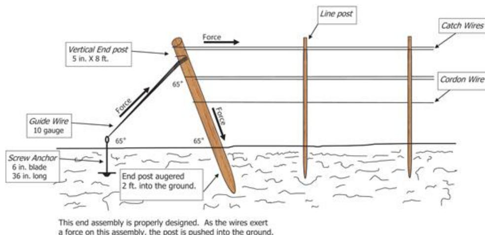
Figure 12. Trellis end post at 65° angle as used in temperate industries (Source: [https://aces.nmsu.edu/pubs/\\_h/H331/](https://aces.nmsu.edu/pubs/_h/H331/)).
