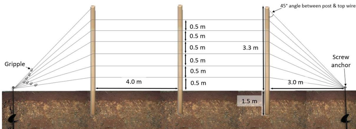
Figure 13. Trellis assembly at 90° angle as used in mango planting systems trial at Walkamin Research Facility
