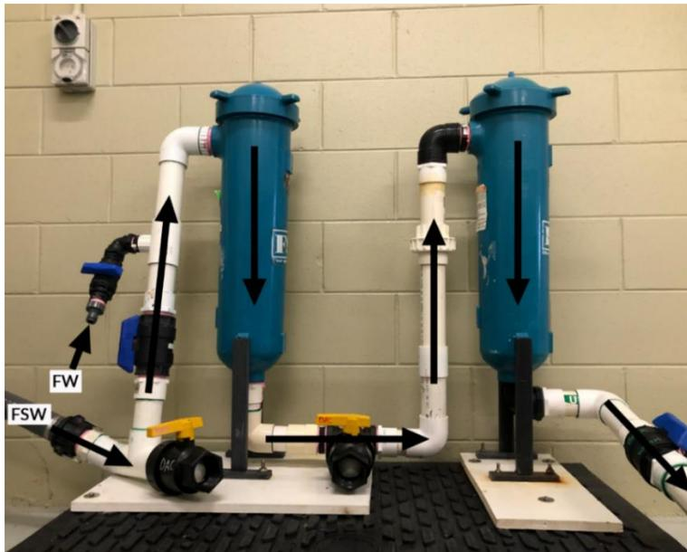
**Figure 1.** Pair of FSI X100 bag filter housings fitted with  $1\ \mu\text{m}$  filter bags placed in series. Arrows indicate the direction of water flow. FSW; filtered seawater and FW; freshwater. FW is used to flush the system when cleaning.
