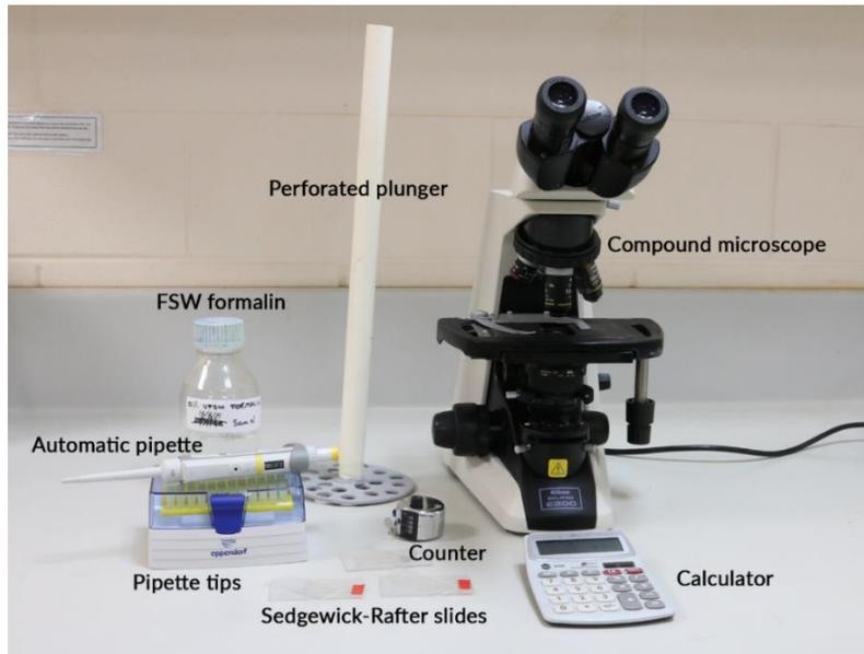
**Figure 10.** Equipment to sample, measure and assess larvae.
