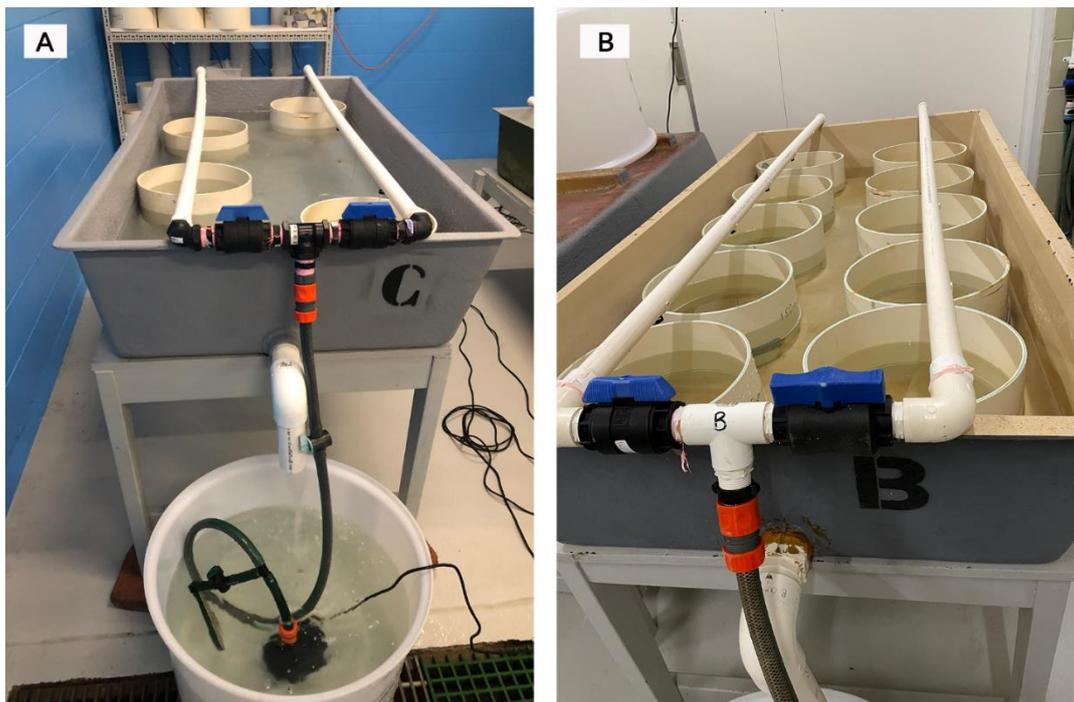
**Figure 18.** (A) Recirculating downweller system for settlement and (B) close up of spray bars and holding screens in the downweller system.
