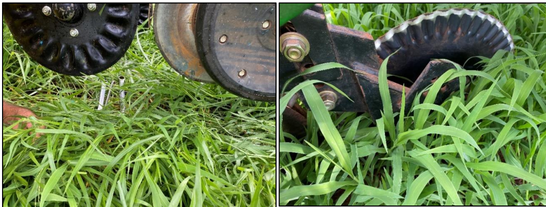
Photo. 5. 1 Left- Bubble coulters and Right - Fluted coulters
