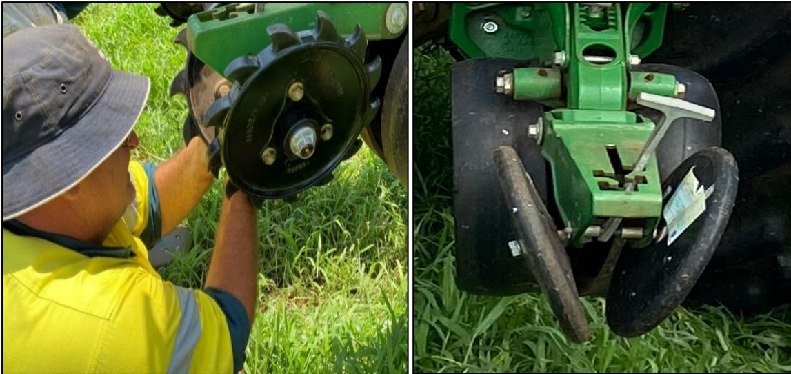
Photo. 5. 2 Left - Spiked press wheels and Right - Rubber press wheel
