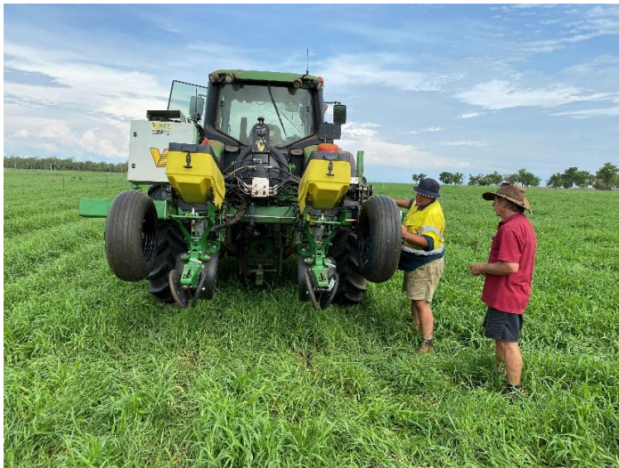
Photo. 5. 3 Stephan Frahm from Vanderfield-RDO, above left, supplied a two row planter with various planter configuration's, monitoring sensors and assisted with planting set up, changing with a number of different coulters and press wheels. Seen here with planter set up.
