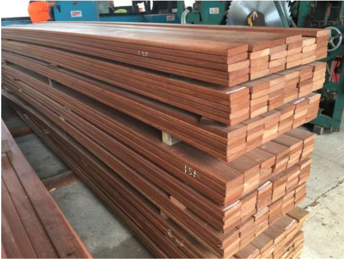
Cape York Timber sawn product using Darwin stringybark ( Eucalyptus tetradonta ), Cape York, Queensland
