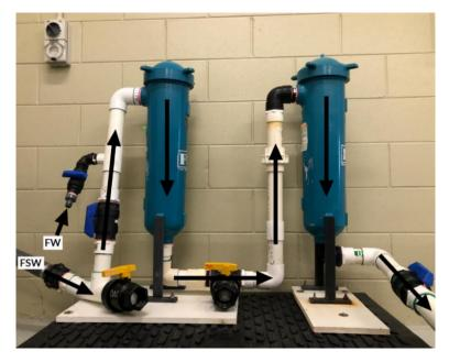
**Figure 1**. Pair of FSI X100 bag filter housings fitted with 1  $\mu$ m filter bags placed in series. Arrows indicate the direction of water flow. FSW; filtered seawater and FW; freshwater. FW is used to flush the system when cleaning.
