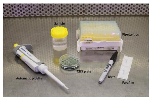
Figure 13. Equipment for Vibrio testing inside laminar flow cupboard.
