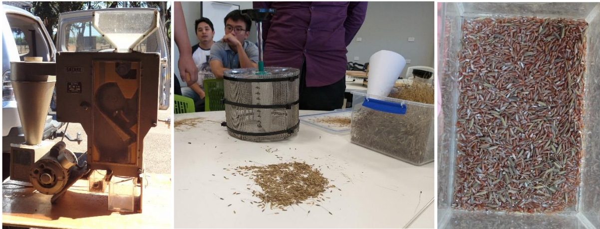
Figure 8.2 Research-scale Satake Testing Husker (left), native rice thresher (middle) and milled wild-harvested native Australian rice (right). Photos: Penny Wurm
