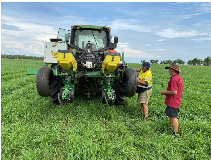
Photo. 5. 3 Stephan Frahm from Vanderfield-RDO, above left, supplied a two row planter with various planter configuration's, monitoring sensors and assisted with planting set up, changing with a number of different coulters and press wheels. Seen here with planter set up.
