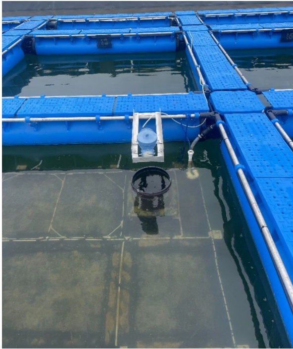
Figure 8. Arvo-Tech feeder installed on a large enclosure. Feeder undergoing testing.
