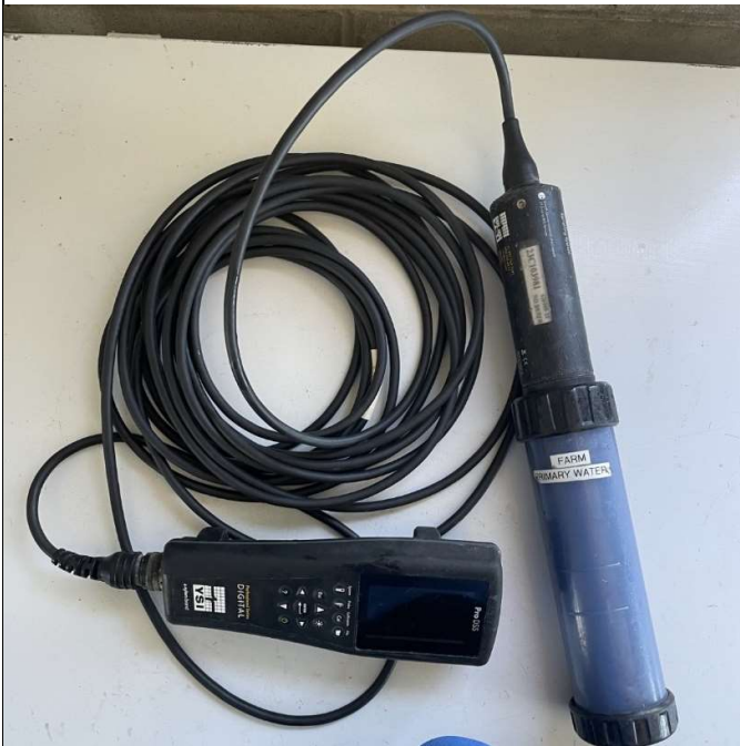
Figure 2. Primary Water and Growout ProDSS Water Quality Probe
