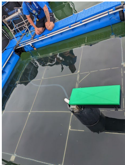
Figure 7. Belt feeder installed on a large enclosure (left). Close-up of a feed tube and the clock system of a belt feeder (right), which activates the belt to automatically provide three feed rations during a period of 12 hours.
