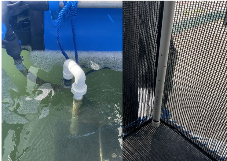
Figure 5. PVC/POLY manifold assembly to ensure water flow in enclosures used for TRL grow-out.
