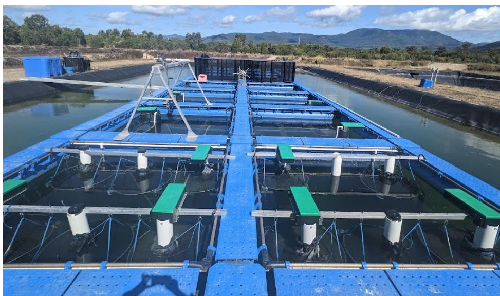
Figure 6. Belt feeders installed to medium size enclosures in the grow-out system.
