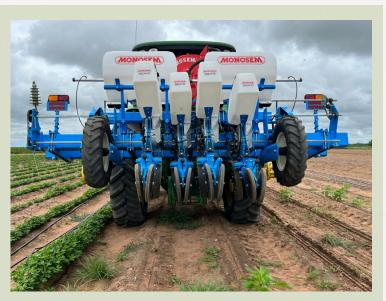
*Figure 1:* Monosem precision planter used for sowing Kalonji on 30 cm row spacing in Emerald, QLD.
