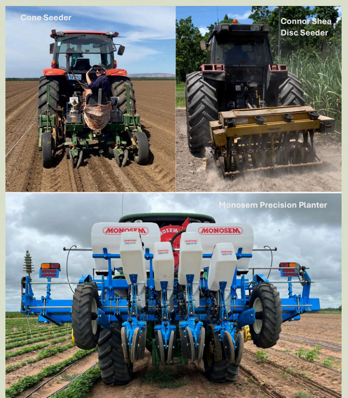
Figure 2: Planters used for sesame. Top Right: Cone seeder sowing four rows in Kununurra, WA; Top Left: Connor Shea disc seeder sowing four rows in Tully, QLD; and Bottom: Monosem precision planter sowing four rows in Emerald, QLD.
