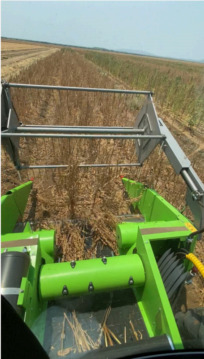
Figure 13: Heading a mature dry sesame crop with a plot header with a platform front.
