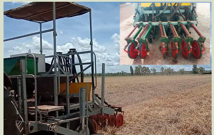
Figure 1: Direct drilling of sesame into Sabi grass stubble using a cone seeder in summer 2022-23 in Katherine, NT.
