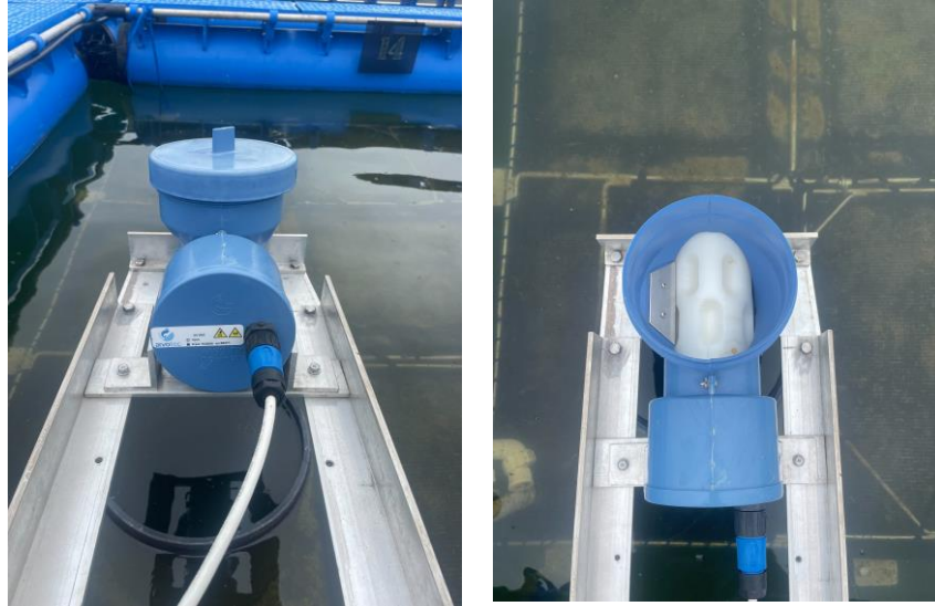
Figure 12. Arvo-tec feeding system installed to a large enclosure in the second grow-out system to increase accuracy in feeding time and volume.
